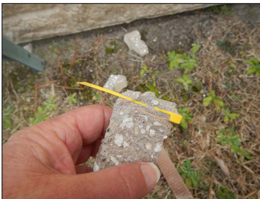
NO. 62 - SPALLED WALL PANEL ON THE SOUTH SIDE OF COLUMN 13NM - EMBEDDED ZIP TIES
