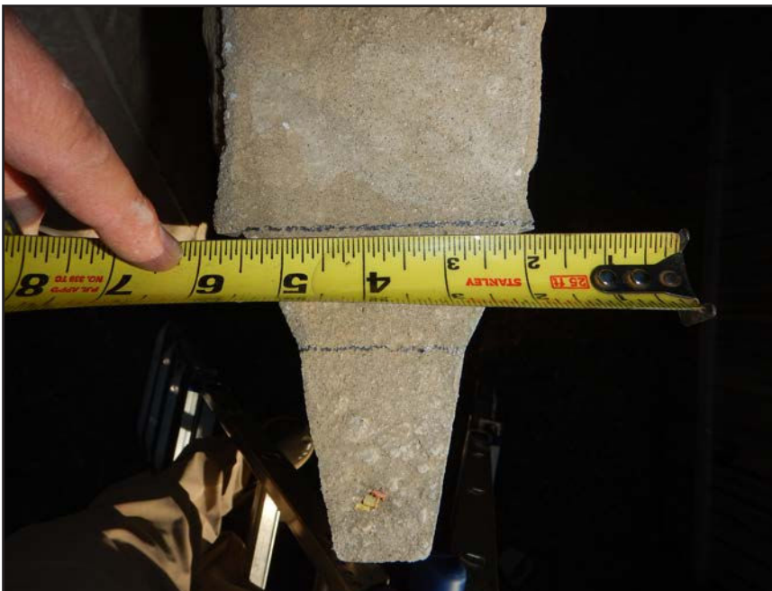
NO. 28 - STORED EXCESS WALL PANELS - TYPICAL TONGUE DIMENSIONS
