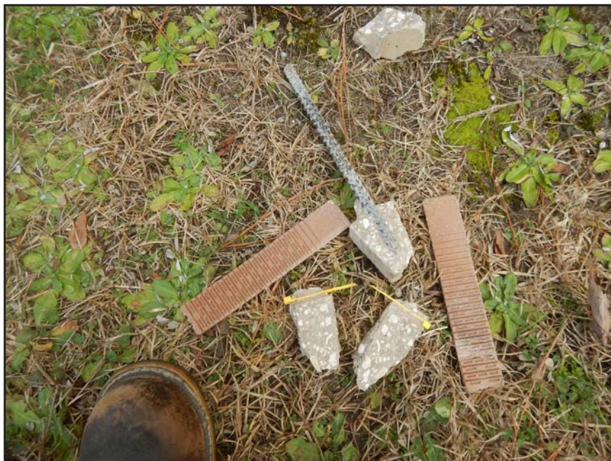
NO. 60 - SPALLED WALL PANEL ON THE SOUTH SIDE OF COLUMN 13NM - TONGUE REINFORCING DOWEL WITH INADEQUATE CONCRETE COVER
